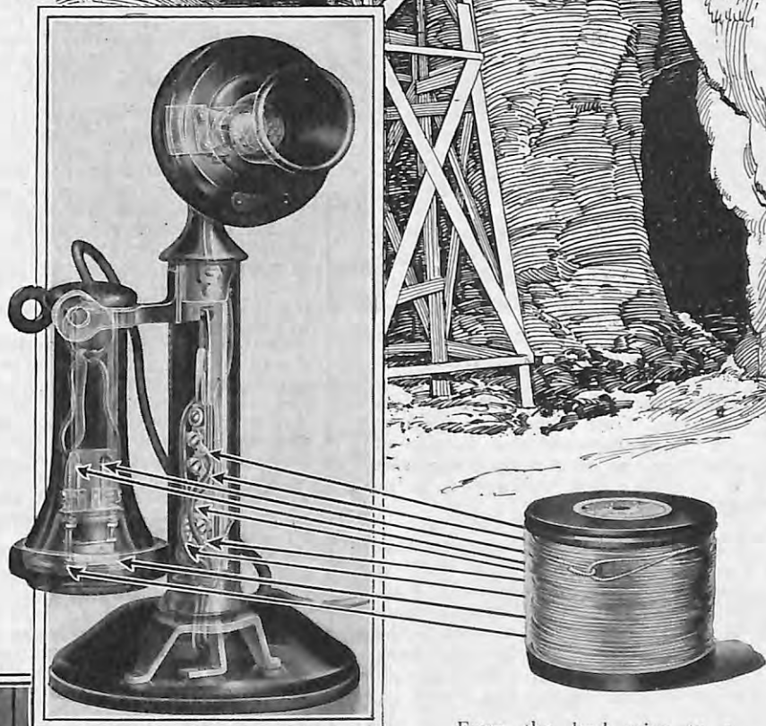
From the lead mine to a spool of solder—for permanent electrical connections between many small telephone parts.
