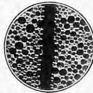
ORDINARY LATHER Photomicrograph of lather of an ordinary shaving cream surrounding single hair. Large dark spots are air—white areas are water. Note how the large bubbles hold air instead of water against the beard.
