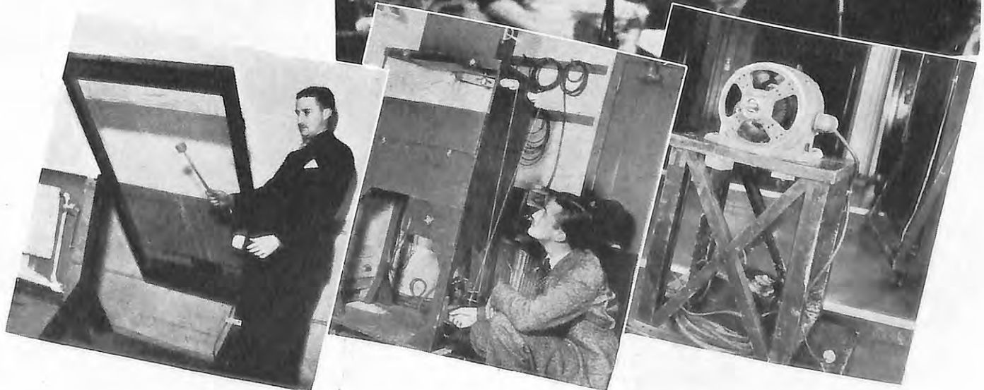
Below, from left to right: Ray Kelly, NBC's sound effects chief, makes thunder with a window screen, and next, Kelly testing his rain-making machine, which works by dropping rape seed on a circular disk. Last: The wind machine, which can produce either a zephyr or a gale
