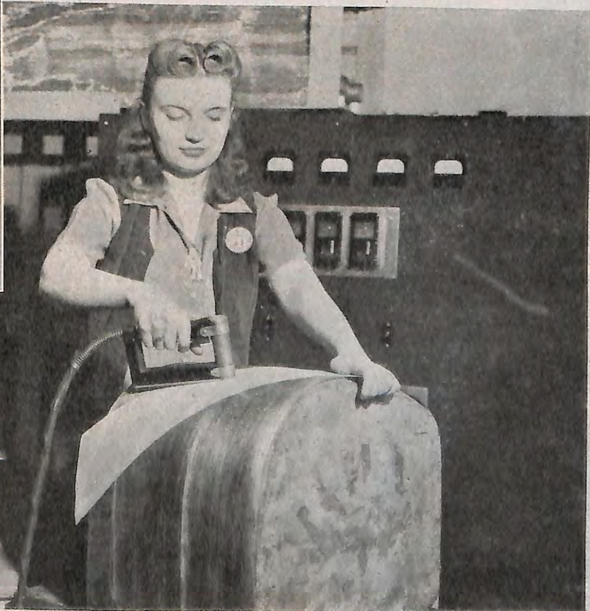
Below: RCA's "radio nail" gun which was developed primarily for the temporary bonding of thin veneers of wood.
