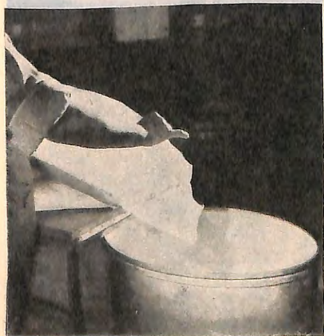
Batching of dried tablet granulation.
