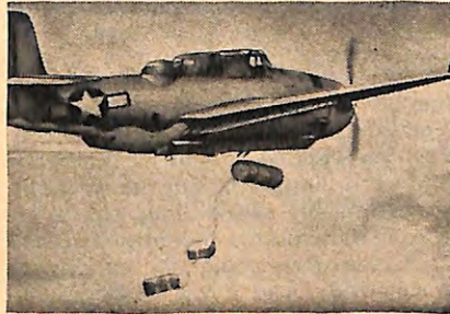
1 A rescue job for the AR-10 assembly! Dye marks in the ocean lead this searching Navy "Avenger" to a shipwrecked crew. Out of the bomb bay goes the 240-yard train of packages.
