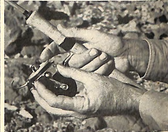
For the next step, flip the pickup arm of your spinning reel out of the way.
