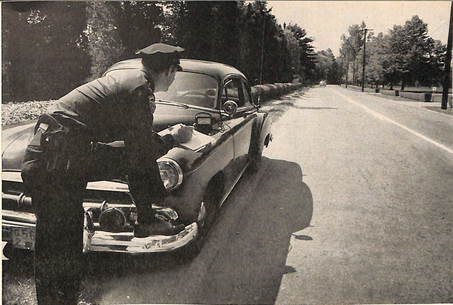
Here traffic is being checked for traffic and density by a Speed Meter on Connecticut's famed Merritt Parkway.
