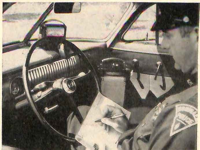
You don't see the policeman. Police watch the dial which registers your speed from inside the car. Radio telephones your license number and car description ahead. Surprised speeder then is stopped and handed a ticket.
