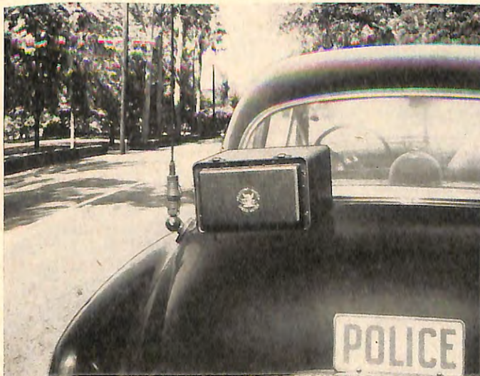
Beware the black box. Placed unobtrusively on a car fender, or on the ground, the Speed Meter sends out microwaves that measure very exactly speed of your car and it takes less than 3/10ths of a second to do it.
