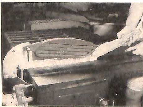
NARROW OR SMALL PIECES (A) should always be ripped with the aid of a push stick, which has a notch cut at about 30° to its long dimension, and a handle shaped to fit the hand. Note how the splitter helps hold work against fence.
