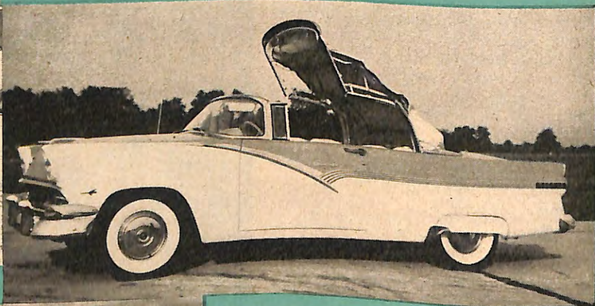
Above: A Ford Division first for '56 is an automatic convertible top latch. The symbol on front fender indicates that this top line Fairlane has modified version of last year's Thunderbird engine. Ford still produces an economy 6-cylinder engine; V-8 power ranges from 173 to 202 horsepower. Author tried Ford's safety belts (above left) and found them to give increased feeling of security. On this convertible Fairlane the sun visors are also padded for impact safety.
