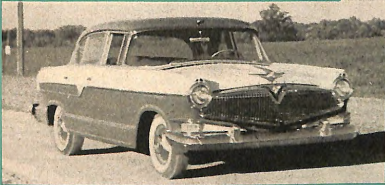
Left: Hudson Hornet was put through its paces on Burlington, Wis., proving grounds. New engine puts out 220-horsepower and performance, comfort and roadability are on par with the field. Hornet shown here negotiating strip of concrete test washboard surface at good clip.
