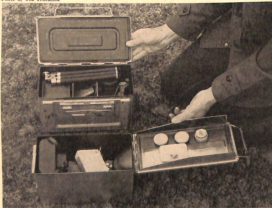
Two ideas for waterproof, dust-proof camera boxes made from 50-caliber ammunition boxes. In the lower one camera, flash attachment, filters, lens shade, cable release and self-timer are held in place by brackets, screws or wing nuts. The upper box is divided by partitions held in place by glue. A twin-lens reflex is in the left compartment, filters, film and meter in the middle one, 35 mm miniature and its telephoto in the right. The tripod lies across the top.
