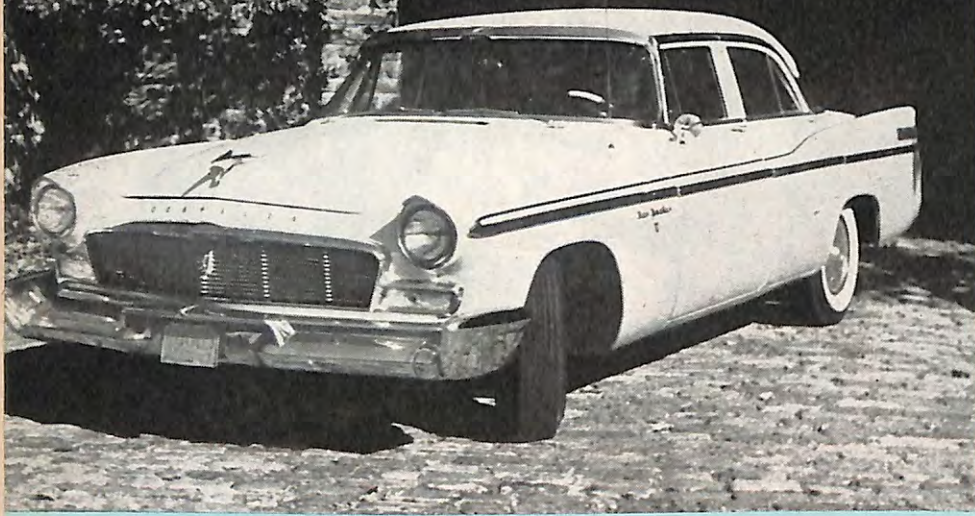
Above: Chrysler New Yorker—on a 126-inch wheelbase, the Chrysler cars show the evidence of air age influence with high swept tail fins. Power ranges from 225-horsepower with the Windsor to 280 in the New Yorker. New styling includes bumpers, rear fenders, grille, chrome trim which is designed with view to practical two-toning.
