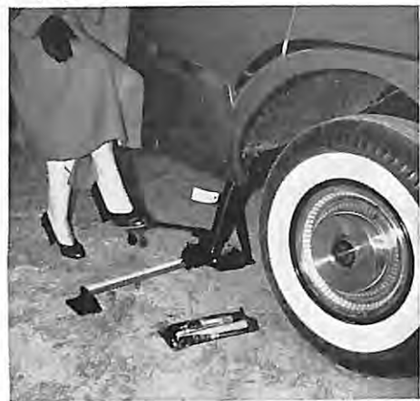
Buick's new foot operated jack can be placed in position beneath side frame rails and car hoisted easily by foot pressure. This represents an intelligent adoption of a feature long used on European cars.
