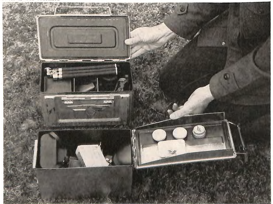
Two ideas for waterproof, dust-proof camera boxes made from 50-caliber ammunition boxes. In the lower one camera, flash attachment, filters, lens shade, cable release and self-timer are held in place by brackets, screws or wing nuts. The upper box is divided by partitions held in place by glue. A twin-lens reflex is in the left compartment, filters, film and meter in the middle one, 35 mm miniature and its telephoto in the right. The tripod lies across the top.
