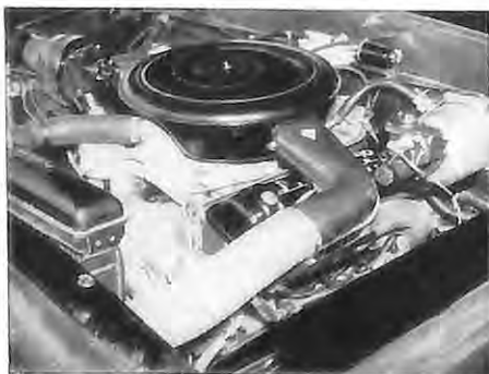
A Lincoln first is the efficient air duct which channels air to the carburetor. A thermostat controls the admittance of cool outside air or warmer under-hood air to assure better fuel-air mixture. This is an exclusive feature. (Photo by: Joe Farkas, Ford Photo Section)
