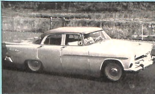
Plymouth Plaza features a V-8 engine turning out either 180 or 187-horsepower. Performance addicts can get super-powered Plymouth with 200-horsepower engine. This Plaza is being gunned from a standing start, hence the blurred outline. Savoy and Belvedere models differ chiefly in extent of exterior and interior trim. Buyer can still get reliable 125-horsepower, 6-cylinder engine.
