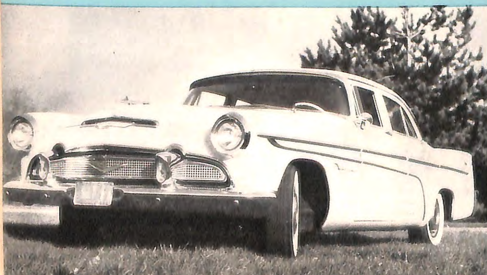
Plymouth Plaza features a V-8 engine turning out either 180 or 187-horsepower. Performance addicts can get super-powered Plymouth with 200-horsepower engine. This Plaza is being gunned from a standing start, hence the blurred outline. Savoy and Belvedere models differ chiefly in extent of exterior and interior trim. Buyer can still get reliable 125-horsepower, 6-cylinder engine.
