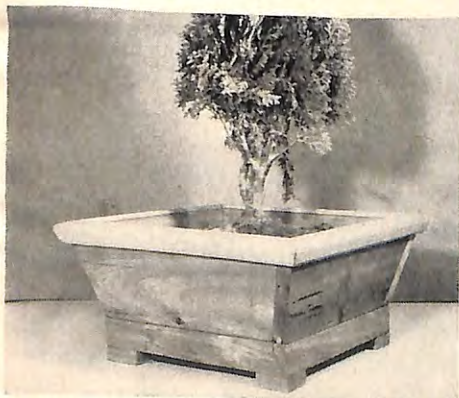
A BOX WITH FOUR SLOPING SIDES calls for care in cutting. These sides were butted and nailed together, one end of each overlapping the next. Four strips were then nailed on beneath, blocks added for feet, and the top edge was trimmed by mitering molding around it.
