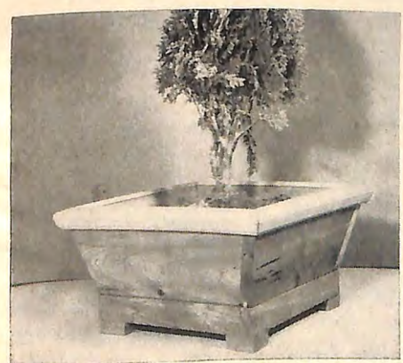
A BOX WITH FOUR SLOPING SIDES calls for care in cutting. These sides were butted and nailed together, one end of each overlapping the next. Four strips were then nailed on beneath, blocks added for feet, and the top edge was trimmed by mitering molding around it.
