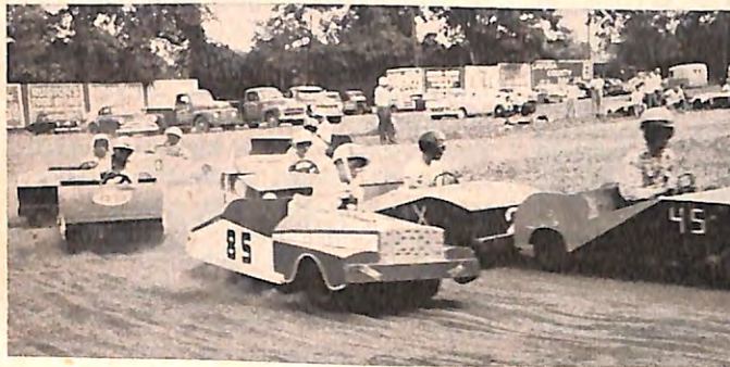
The Auburn, N. Y., Elks Microd Club in action at the former home of the "Can-Am" minor league baseball team, where bi-weekly races draw crowds of from 1,000 to 1,500 spectators. The cars are made of plywood and are powered by gasoline lawn-mower motors, according to M.T.T. specifications. Past State Vice-Pres. Philip J. Conboy is Chairman of the lodge's Youth Committee which sponsors the races.
