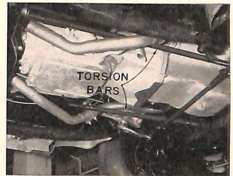
All five Chrysler cars from Plymouth to big Imperial now feature torsion bars rather than traditional coil springs for low and firmer front suspension. Arrows point to the long longitudinal torsion bars which twist with front wheel up-down movements rather than compress.
