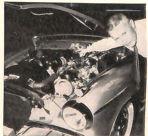
Mike De Blumenthal, Studebaker's Chief Research Engineer, points to the super charger covering carburetor; this pressurizes extra air through carburetor, increasing combustion efficiency of already very warm V-8 engine—gives performance hot enough for anyone to brag about.
