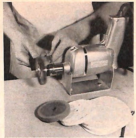
With a drill stand fastened to the workbench, you can clip the drill in for stationary use with a wire brush, polishing pad, buffing or grinding wheel. Handle should be to your left so that the spindle turns toward you.
