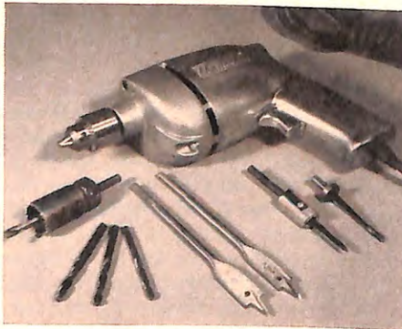
These are home makers. In front of the electric drill, from left to right, are a hole saw, twist drills, wood augers, and two types of wood-screw pilot drills. Small masonry drills (not shown) can also be used in such a drill; big masonry drills require lower speed.
