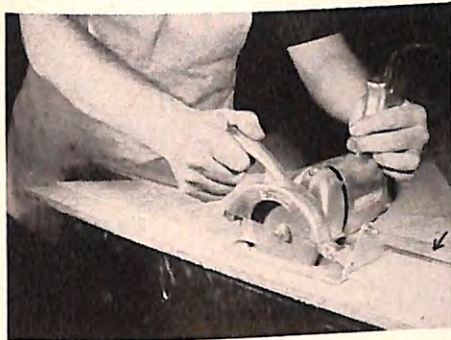
This circular saw attachment bolts to the drill case, making the tool a rigid unit. Feed slowly, and always use a sharp blade. A thin strip of wood tacked to the work (arrow) for the saw shoe to guide along makes more accurate rip cuts than the small metal guide furnished.
