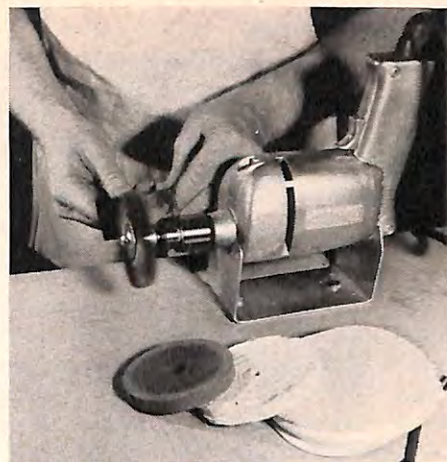
With a drill stand fastened to the workbench, you can clip the drill in for stationary use with a wire brush, polishing pad, buffing or grinding wheel. Handle should be to your left so that the spindle turns toward you.
