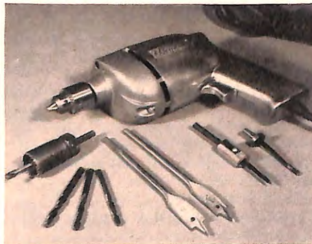
These are home makers. In front of the electric drill, from left to right, are a hole saw, twist drills, wood augers, and two types of wood-screw pilot drills. Small masonry drills (not shown) can also be used in such a drill; big masonry drills require lower speed.
