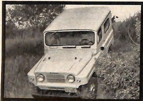
Powerful 135 h.p. waterproof engine climbs up to 65% grades. For added power, transfer case gives 2 or 4 wheel drive in any gear.
