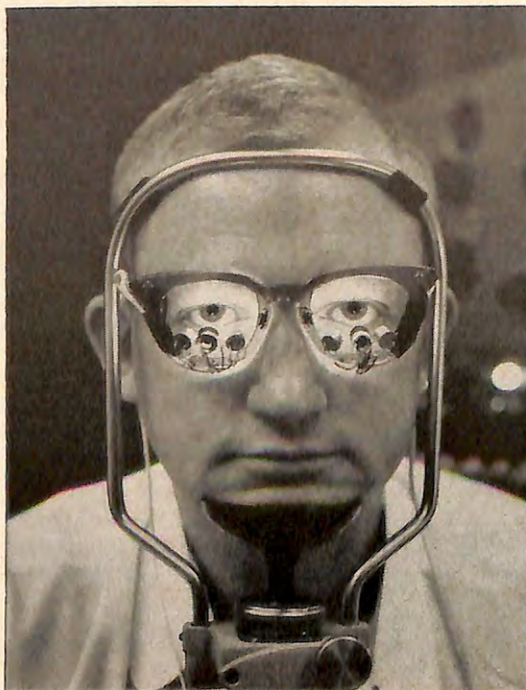
Above: Actual X rays of the on-off medical magnet in use, retrieving a pin blunt end up. Left: These "eye-glasses" are connected to a computer, analyzing eye movements in order to aid in proper diagnosis.
