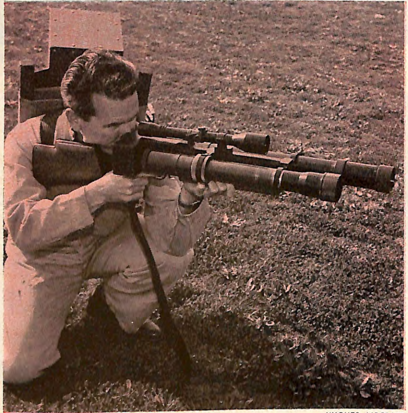
The Colidar Mark II laser device computes range to a target almost instantly. It works essentially like radar, but it is carried and aimed like a rifle.
