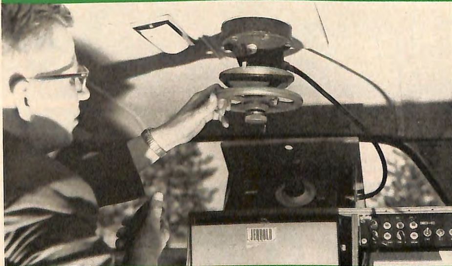
When an illegal signal is reported or discovered, a mobile direction-finding unit seeks out the source. Here the rotating antenna atop the car is actuated to get a bearing.
