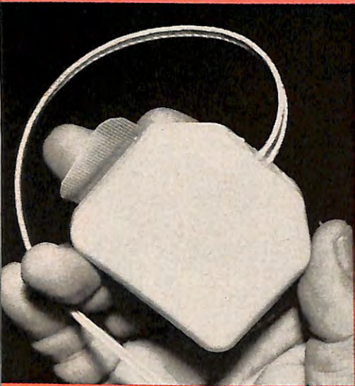
This is a cardiac pacemaker, which, implanted in a patient's chest, maintains the proper heart beat and stretches the life span considerably.
