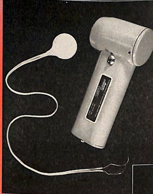
Above, the radiophysiologic bladder stimulator, a boon to paraplegics. It was developed by Dr. Adrian Kantrowitz of Maimonides Hospital of Brooklyn, N. Y., in conjunction with the Avco-Everett Research Laboratory.
