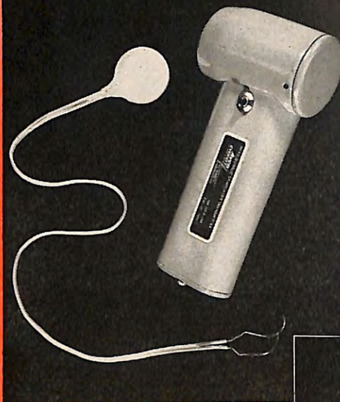
Above, the radiophysiologic bladder stimulator, a boon to paraplegics. It was developed by Dr. Adrian Kantrowitz of Maimonides Hospital of Brooklyn, N. Y., in conjunction with the Avco-Everett Research Laboratory.
