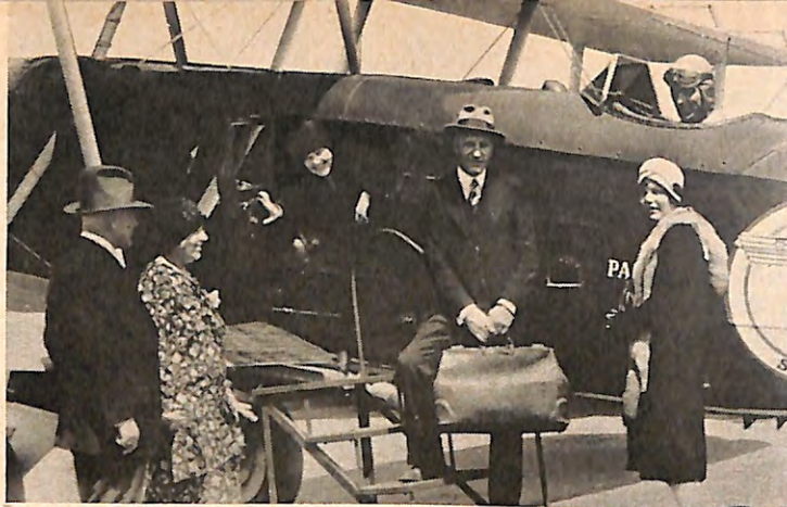
The Boeing 40B-4 biplane carried four passengers beginning in 1926, presumably not in much comfort. It made a then-respectable 110 miles per hour.
