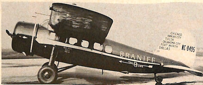
Braniff's Lockheed Vega carried six passengers at 150 m.p.h. back in 1930, on the basis of which the company called itself the "world's fastest airline."
