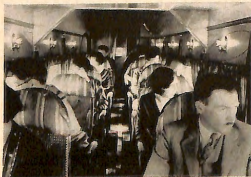
It was the last word in the early '30s—the Ford Tri-Motor, with adjustable wicker seats, individual passenger lights, floor heaters.
