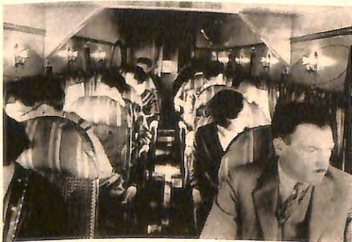
It was the last word in the early '30s—the Ford Tri-Motor, with adjustable wicker seats, individual passenger lights, floor heaters.
