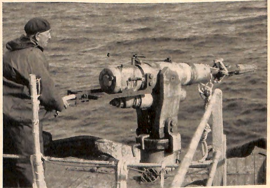
Captain Arne Borgen unlimbers the unwieldy harpoon gun, which fires a 132-pound harpoon that in turn trails a two-inch line through the air.
