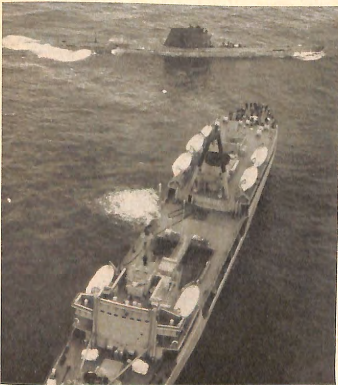
A Soviet submarine of the “Z” class refuels from the tanker Terek ; the Soviet fishing trawlers also could be used as refueling bases.
