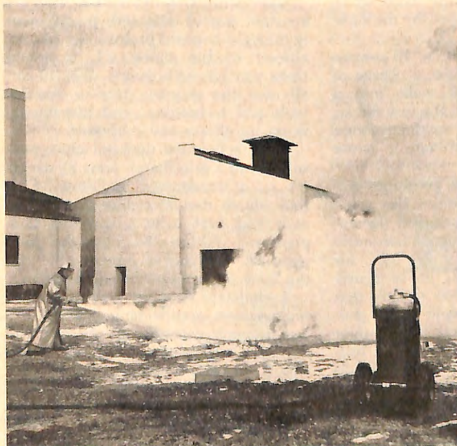
To win UL approval, this wheeled, dry-chemical fire extinguisher must really extinguish a blaze. Technicians check it by starting a 200-square-foot oil fire, then attacking the blaze with chemicals.
