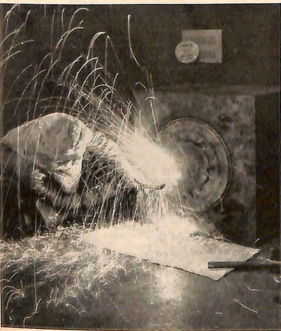
The manufacturer claims this safe is burglar-resistant. UL has already attacked it with sledges, chisels, and drills. Now a technician tries a welder's cutting torch on it.
