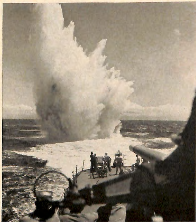
A depth charge explodes off the stern of the U.S.S. Philip during structural tests to determine effect of concussion on ship's hull.
