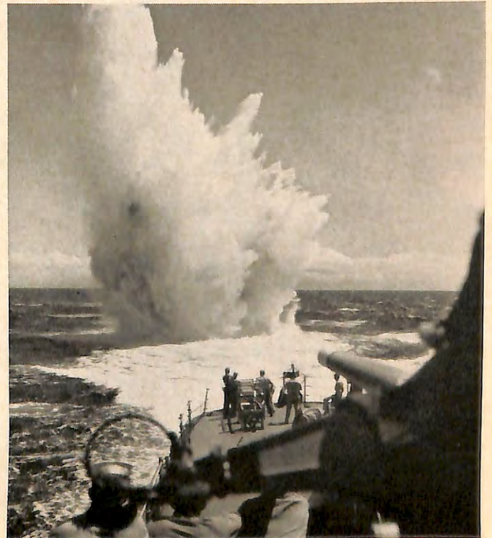
A depth charge explodes off the stern of the U.S.S. Philip during structural tests to determine effect of concussion on ship's hull.
