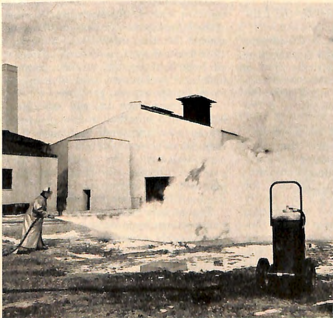
To win UL approval, this wheeled, dry-chemical fire extinguisher must really extinguish a blaze. Technicians check it by starting a 200-square-foot oil fire, then attacking the blaze with chemicals.
