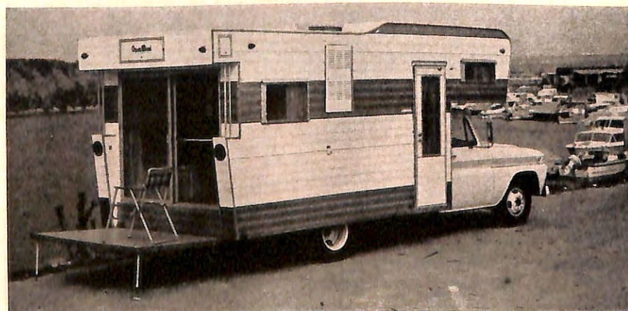
The Open Road camper features a built-in patio that folds up to cover the picture window when on the road, drops to form a sun deck when parked; unit is on a one-ton truck chassis.
