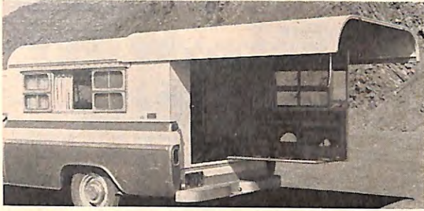
Camper by Pullman has a slide-back canopy and cooking equipment hung in a cabinet on the rear door. Canvas walls can be added to provide more shelter.
