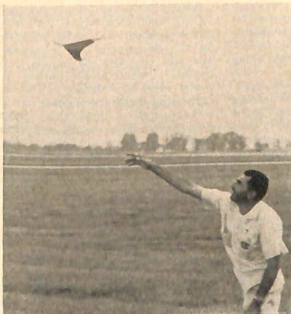
In a preliminary flight, a model rocketeer launches his rocket-powered glider by hand to check its "trim."
