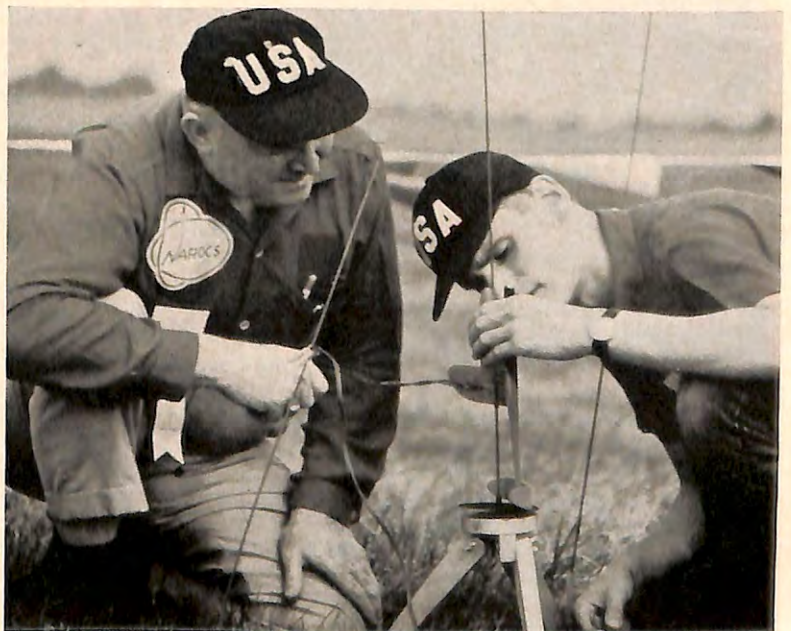
Two rocketeers prepare their boost-glider rocket for launching. This winged model will shoot up like a rocket and drift back like a glider.
