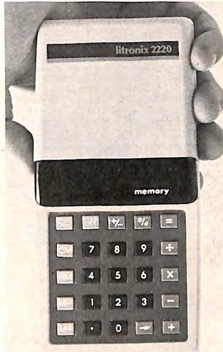
The keyboard on the Litronix was patterned after the expensive Hewlett Packard unit and has a four button, color-coded memory system. Instead of the conventional on/off switch the Litronix has on/off keys.
