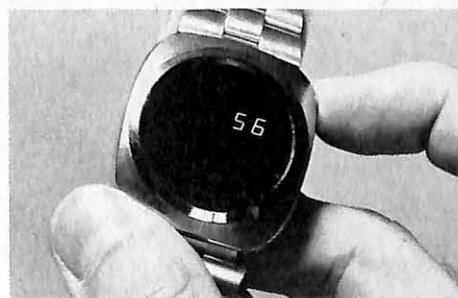
Keep the button depressed and the One Button Digital automatically switches from hours and minutes to display the seconds. Press the button twice and the month and day are displayed.
