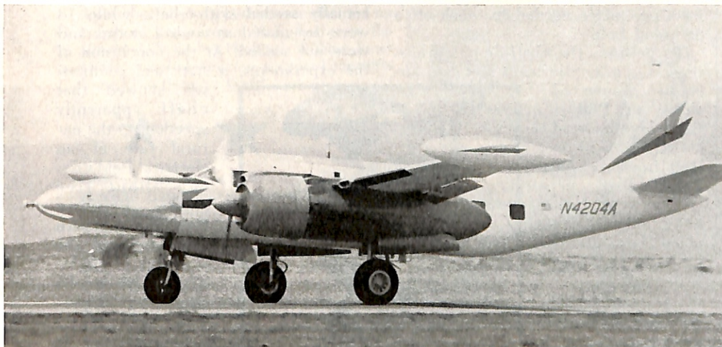
A modified old World War II B-26 bomber readies for take-off on a stormy afternoon in Colorado. It is on a scientific mission to study lightning. The storm-chasing aircraft has two field mills—one on the nose cone and one on top—which monitor atmospheric electric fields. Inside the plane, scientists monitor information from these field mills and an array of other weather-sensitive instruments. Chaff to "seed" the storm and prevent lightning is dropped from a chute at the back of the plane.
