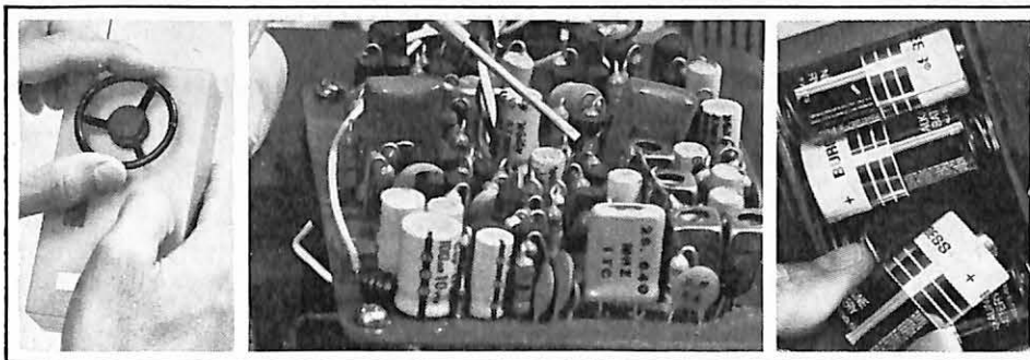
The remote control unit (left) controls the race car's electronics (center). The four "C" cell batteries fit in the underside of the Racer.
