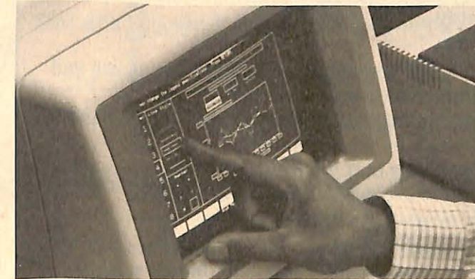
Many systems incorporate innovations that make their computers more "user-friendly" to the novice. The touch-screen shown can make giving the computer instructions as easy as pointing your finger. Photo courtesy of Hewlett-Packard.
