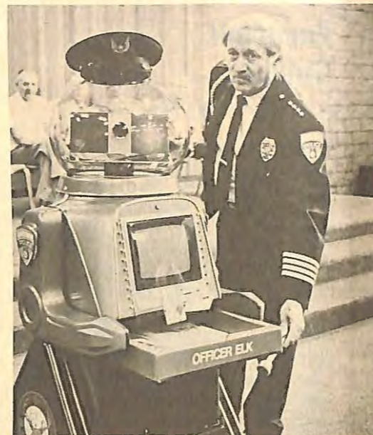
Garden Grove, CA, Elks can be proud of their contribution toward better drug awareness education. Meet Officer Elk, a five foot, four inch tall ARES (Auxiliary Robotic Education System) robot police officer whose unique presence and capabilities will be the focal point of a drug awareness education program for local elementary and junior high school students. Once programmed, Officer Elk, donated by Garden Grove lodge, will be able to conduct a full 40-minute classroom seminar utilizing sophisticated two-way wireless communications, and a video cassette playback unit with 8-track stereo tape player. ER Joe Farquhar has presented Officer Elk with honorary life membership card No. 1952 (the lodge's number) and Garden Grove Mayor Jonathon Cannon has duly sworn the robot into the Police Department and has assigned him badge No. 1952 in honor of his donors. Chief of Police Frank Kessler, a member of Garden Grove lodge, demonstrates Officer Elk's capabilities.
