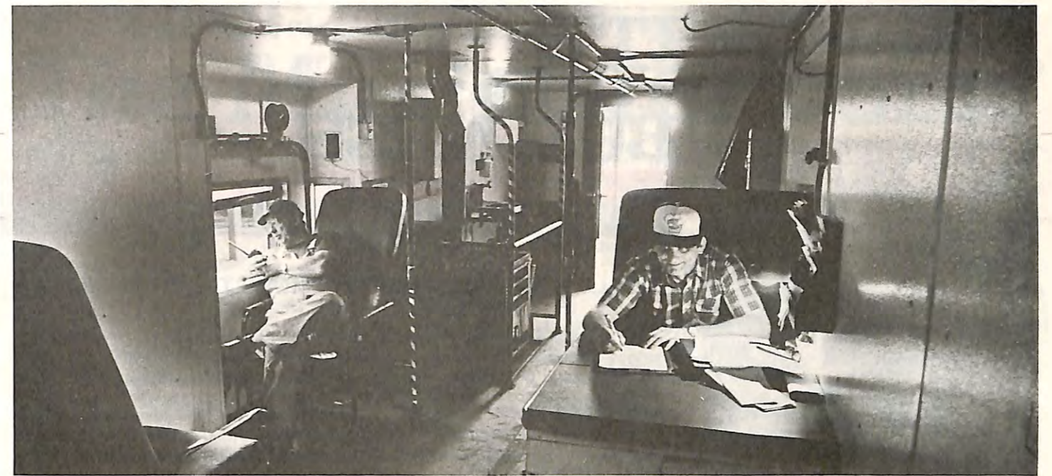
This is the sparse interior of a Chicago and North Western Railway caboose. The conductor attends to paperwork while the brakeman watches the freight cars ahead for possible wheel problems.
