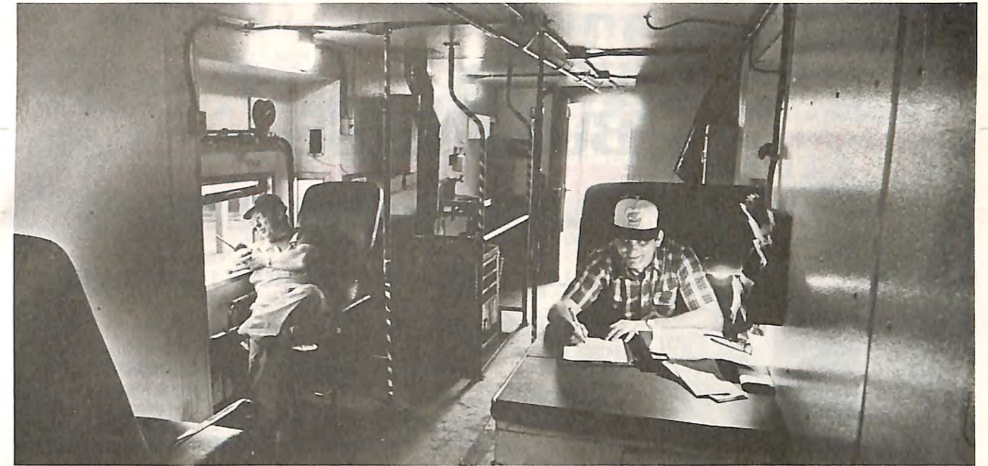
This is the sparse interior of a Chicago and North Western Railway caboose. The conductor attends to paperwork while the brakeman watches the freight cars ahead for possible wheel problems.
